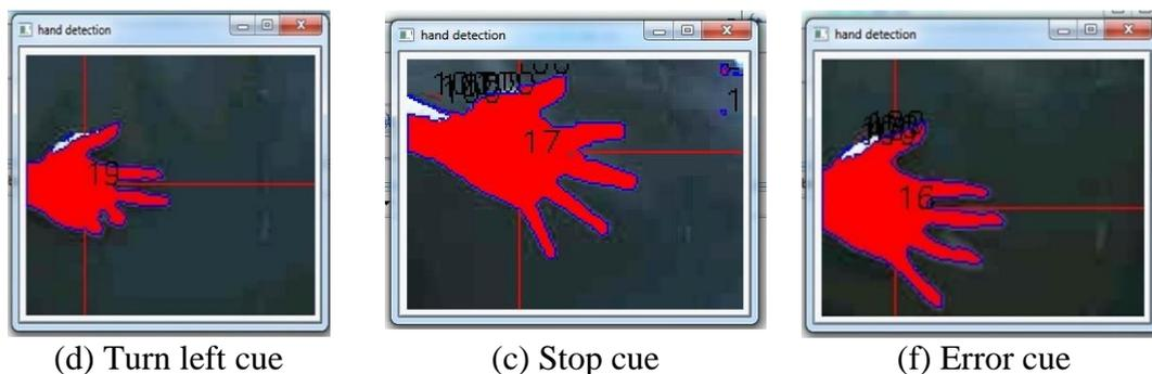
FIGURE 6. Finger cues to drive robot motion.
