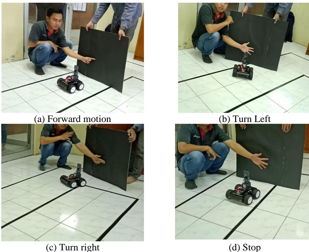
FIGURE 7. Finger cues and robot motion during experiment.
